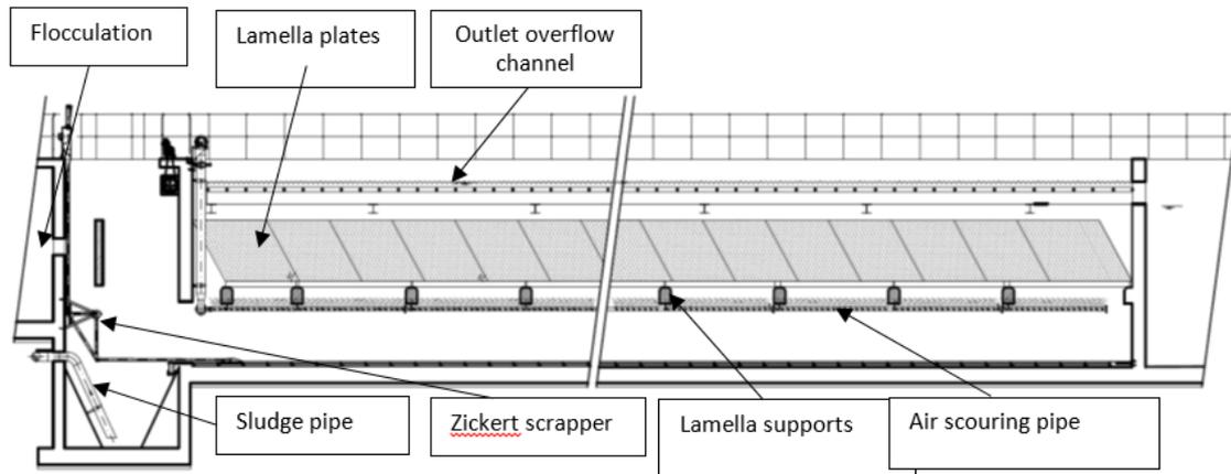
**Figure 5-13:** Lamella settlers proposed configuration
