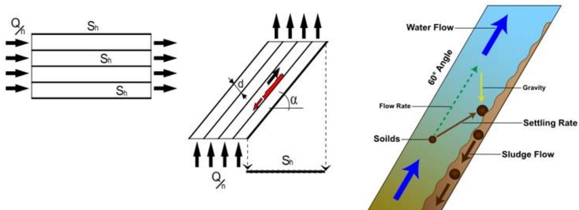
**Figure 5-9:** Diagram of a lamella clarifier basic operation
