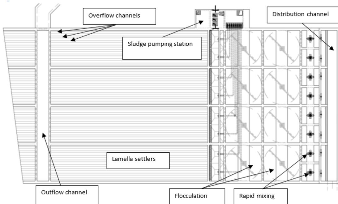
**Figure 5-12:** Chemical enhanced sedimentation – lamella settlers
