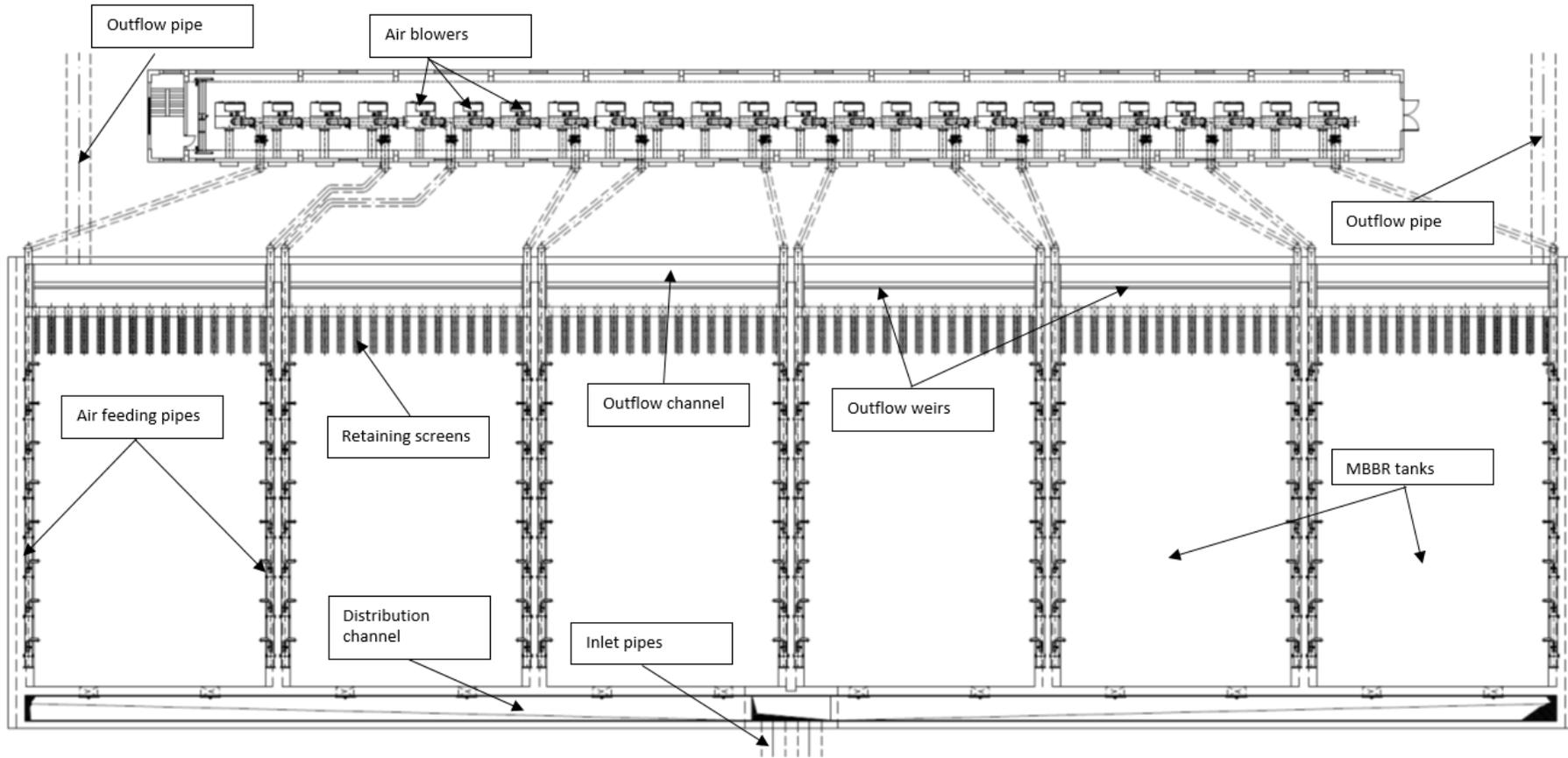
Figure 5-11: MBBR tanks proposed configuration
