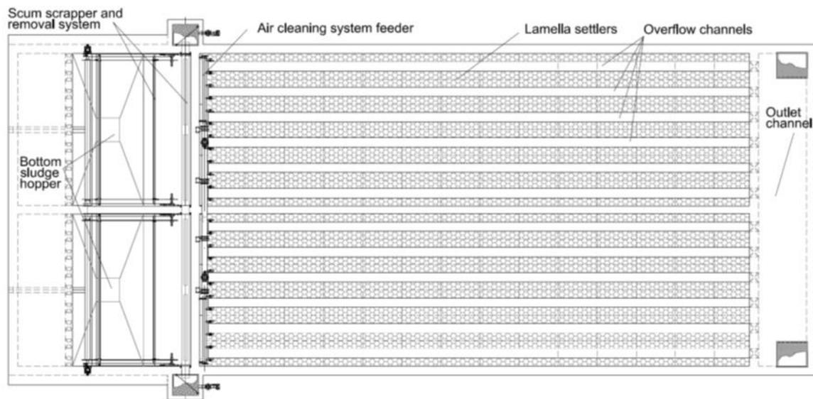
Figure 5-10: Primary sedimentation tanks proposed (with lamella settlers)
